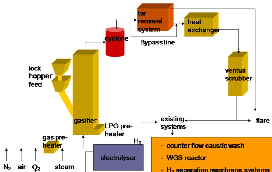
Fig.9. O<sub>2</sub> blown FB gasification system in CRL
