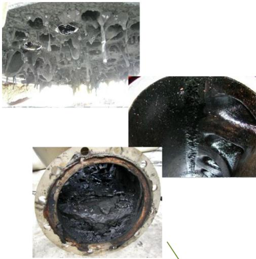
*Fouling and plugging caused by biomass tars: heat exchanger, gas engine, pipes.*
