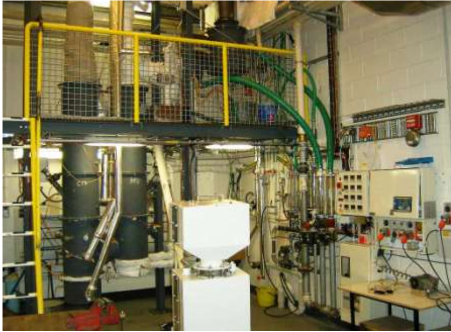
Fig. 8. 100 kW biomass gasifier in CAPE of UoC
