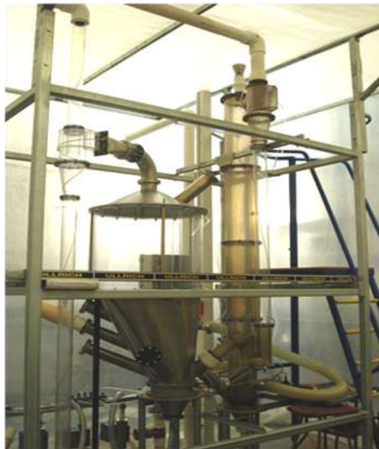
Fig. 9. Cold and transparent DFB model in UoC
